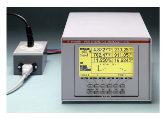
The Infratek 101A single- and three phase Power Analyzer is an economical solution for many measurement applications.
